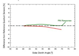
Mean **cosine response** of seven Apogee SQ-500 quantum sensors. Cosine response was calculated as the relative difference of SQ-500 quantum sensors from the mean of replicate reference quantum sensors (LI-COR models LI-190 and LI-190R, Kipp & Zonen model PQS 1). The red data are AM measurements; the green data are PM measurements.
