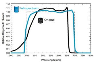
Mean **spectral response** measurements of six replicate Apogee SQ-100 and SQ-500 series quantum sensors. Spectral response measurements were made at 10 nm increments across a wavelength range of 300 to 800 nm in a monochromator with an attached electric light source. Measured spectral data from each quantum sensor were normalized by the measured spectral response of the monochromator/electric light combination, which was measured with a spectroradiometer.
