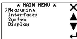
Four icons on the right are used to navigate through the menu. Icons ▲ and ▼ moves the cursor up or down, X leaves the menu or decreases the menu level. The icon ← increases the menu level.
