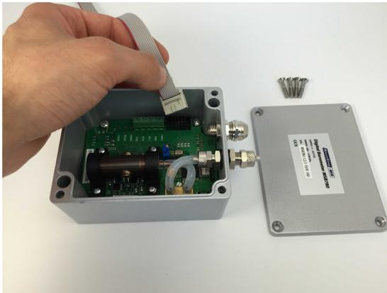
**Figure 8:** Connecting the service cable to the service connector of the MSB780
