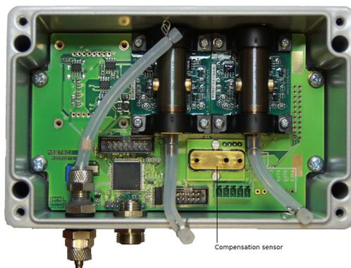
**Figure 4:** MSB780X - checking / exchanging compensation sensor
