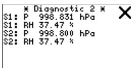
Diagnostic 2 also helps solving problems, it displays pressure from each transducer. If you have version MSB780X with more transducers, there are more pressure values displayed. The example shows case with two pressure transducers.
